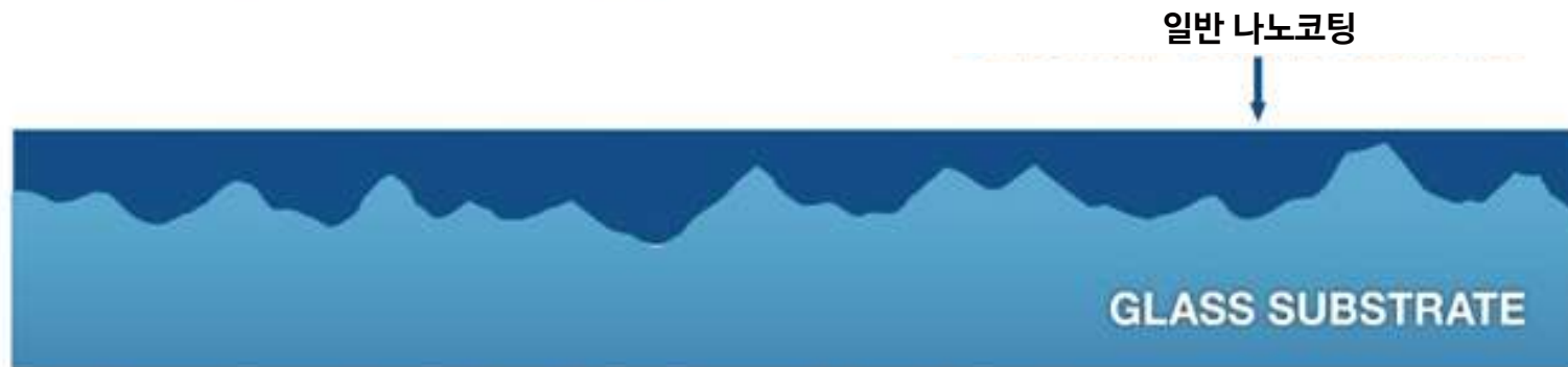
Fig 1. Competitive products that fill in the hills and valleys of the glass
